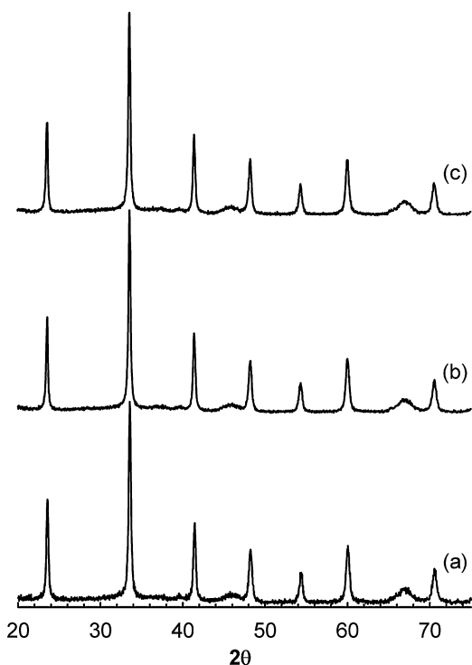
Fig. 8. X-ray diffraction patterns corresponding to P20C/Al 2 O 3 -La 2 O 3 reduced at 900 °C and after passivation (a), reoxidation at 200 °C (b) and reoxidation at 500 °C (c).
